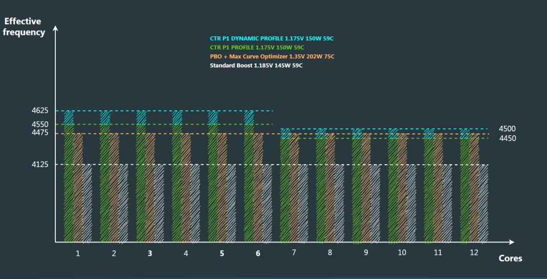
In this example, we see that Cinebench R23 is not putting too much load on the CPU, and so CTR has determined that it is safe to increase the frequency for each CCX. **+75 MHz for CCX1 and +50 MHz for CCX2**. The final difference (V/F) between PBO + Max CO and CTR in this example was **17.2% (3.31 vs 3.88)**. You can see a demonstration of the dynamic P1 under different loads <u>here</u>.
